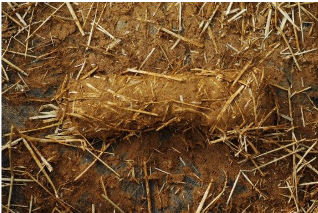
Some sticky, straw-heavy cob — perfect for finishing the top of the cob arch
